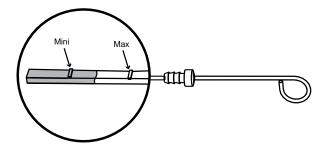
If the level is too low, remove the oil filler plug and add oil slowly. Wait few minutes before checking the oil level to let the oil drain down to the oil pan.
