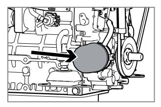
**1.** Remove the oil filter with a filter wrench. Turn the filter counter-clockwise. Remove the gasket.
