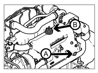
**1.** Turn the coolant filler cap **B** slowly to the first stop and let any pressure escape from the system then remove the cap.
