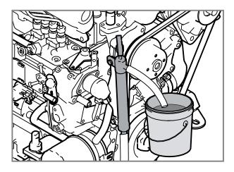
**4.** Suck out all the oil using the oil drain pump. Remove the drain hose and lock the pump.
