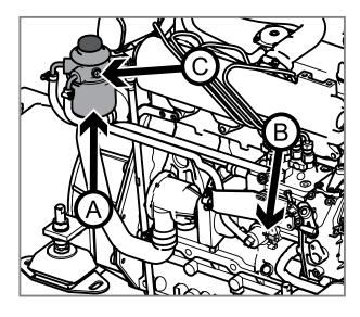
**1.** Close the fuel cock. Clean the filter bracket. Put a plastic bag over the filter to prevent leakage on the engine.
