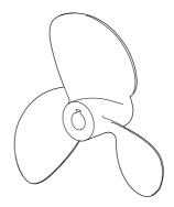
The performance of your engine will be critically affected by the choice of propeller, as an incorrect choice could also damage the engine. Engine speed depends on the propeller size and boat load. If engine speed is too high or too low for good engine performance, this will have an adverse effect on the engine.
