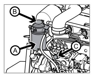
**1.** Close the fuel cock. Clean the filter bracket. Put a plastic bag over the filter to prevent leakage on the engine.
