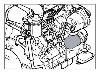
**1.** Remove the oil filter with a filter wrench. Turn the filter counter-clockwise. Remove the gasket.
