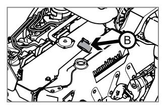
**1.** Turn the coolant filler cap **B** slowly to the first stop and let any pressure escape from the system then remove the cap.
