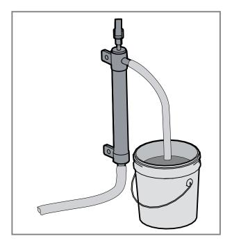
**4.** Suck out all the oil using the oil drain pump. Remove the drain hose and lock the pump.
