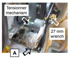
**5.** Check the tension after few hours of operation.
