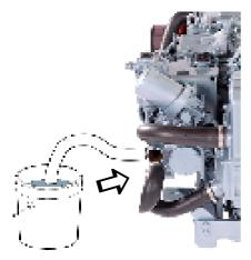
**4.** Check that no one is in the vincinity of the engine, the propeller and the exhaust outlet. Put the lever in neutral and start the engine.
