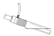
If the boat is equipped with a braided-type stuffing box, check the system's tightness. As this system is not absolutely tight, it is normal that a slight amount of water passes through the stuffing box. Correct operation is characterized by a drop-by-drop water intake. If too much water comes in, stop the engine and contact your Nanni dealer as soon as possible.
