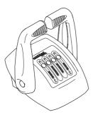
On most boats, the control lever controls both the engine rpm and the gear shift (ahead / astern). However, some boats can be equipped with a separated shift command.
