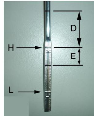
When the engine is fitted inclined, the oil dipstick must be modified to avoid problems of aspiration by the oil pump. See the table enclosed for modification level in rod oil. Increase level D or decrease the level E, starting off of level H of the original oil dipstick.
