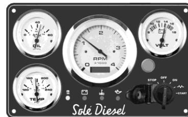
Allow to run at low speed for 4 or 5 minutes and place the gearbox remote control lever in the neutral position. Turn the starter key to “STOP”
